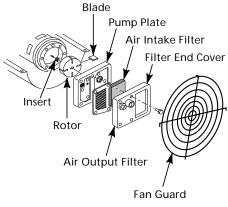
Figure 18 - Rotor Location
